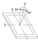
Inspction should be performed withen  $\phi$  ( $\phi$  is usually 30°) from Z axis to each X and Y axis. Inspection distance of any direction withen  $\phi$  must be kept 30 $\pm$  5cm to the display surface.
