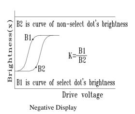
Contrast Ratio (K)=  $\frac{\text{Brightness of non-selected dot (B2)}}{\text{Brightness of selected dot (B1)}}$
